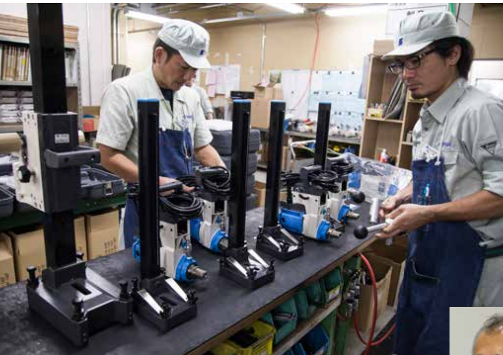
Above assembly of the Shibuya drill systems.
